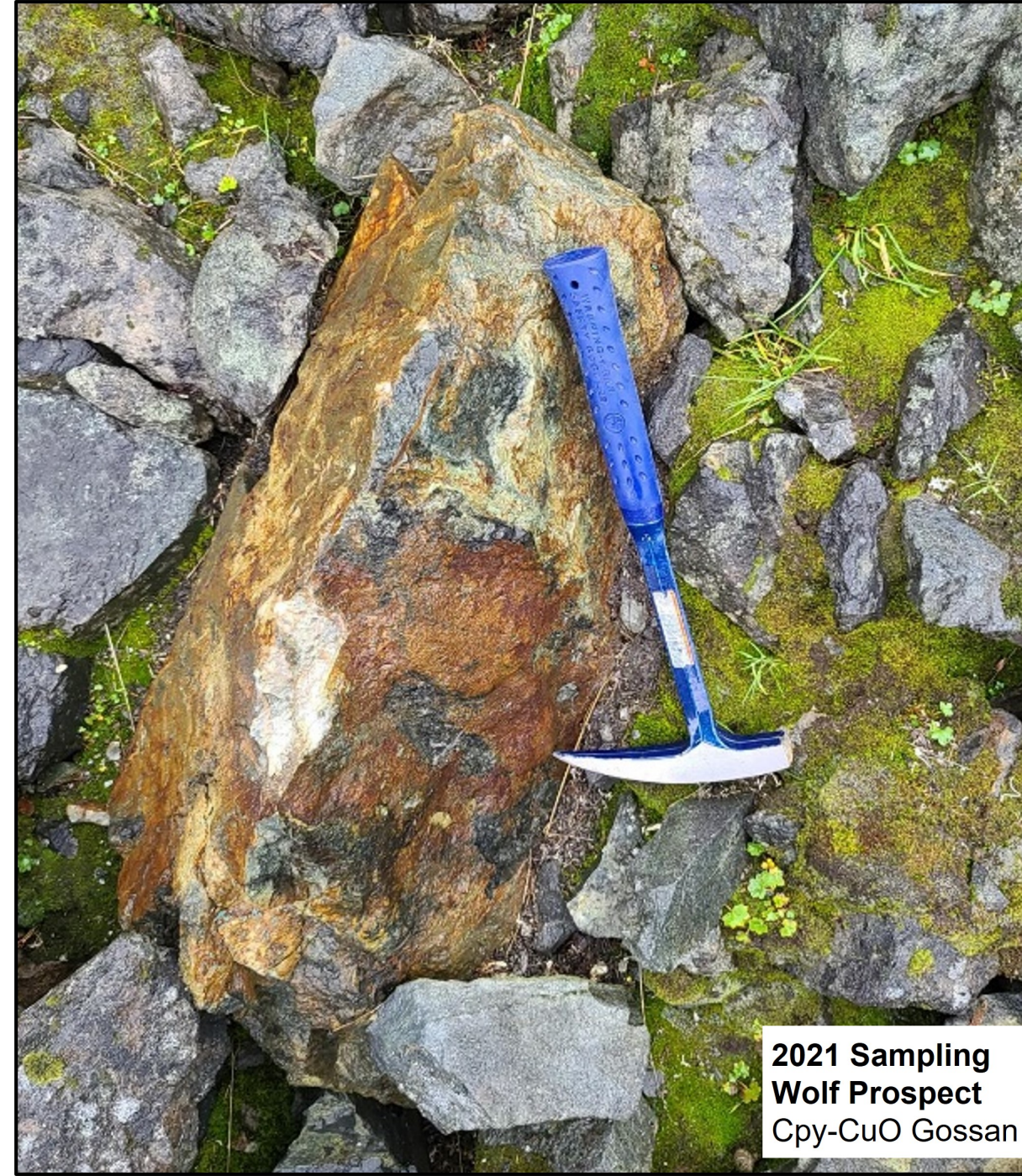
2021 Sampling Wolf MINFILE Epidote clast replacement with CuO veinlet
