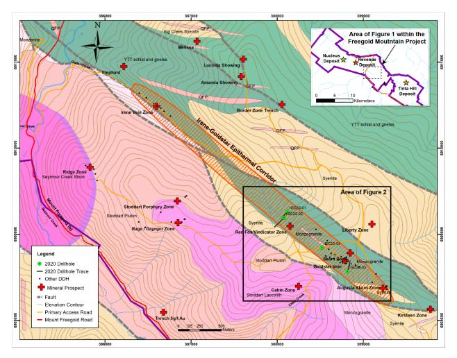
**Figure 1**: Plan Map of the 3.7 kilometre long Irene-Goldstar Epithermal Corridor (outlined in red hatch) located in the Mount Freegold Area between the Tinta Hill and Revenue Deposits.
