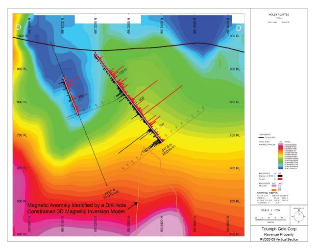
Figure 7 (Cross-Section D to D' in Figure 5): Cross-section of RVD20-03 displaying measured down hole magnetic susceptibility in black and gold grade in red. The magnetic anomaly identified by the Drillhole-Constrained 3D Magnetic Inversion Model (outlined in orange) was intersected where expected, after a significant fault structure at approximately 275 metres downhole.
