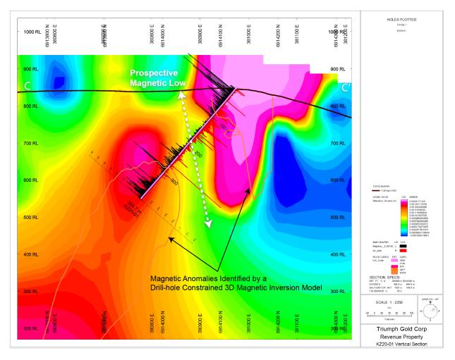
**Figure 6** (Cross Section C to C' in Figure 5): Cross-section of KZ20-01 displaying measured down hole magnetic susceptibility in black and gold grade in red. Two magnetic anomalies were identified in the Keirsten Zone by a Drill-hole Constrained 3D Magnetic Inversion Model (outlined in orange). The anomalies were found where expected, bound by significant fault structures. Mineralization increased between anomalies.
