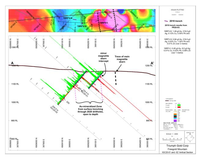
Figure 3 (Cross Section A to A' from Figure 2): Cross-section through IGC20-01 and IGC20-02 displaying high grade gold and silver related to massive magnetite of the oxidized Skarn Zone at approximately 30 metres depth in IGC20-01, as well as newly drilled gold, silver, and base metal mineralization within the Irene-Goldstar Corridor in both IGC20-01 and IGC20-02
