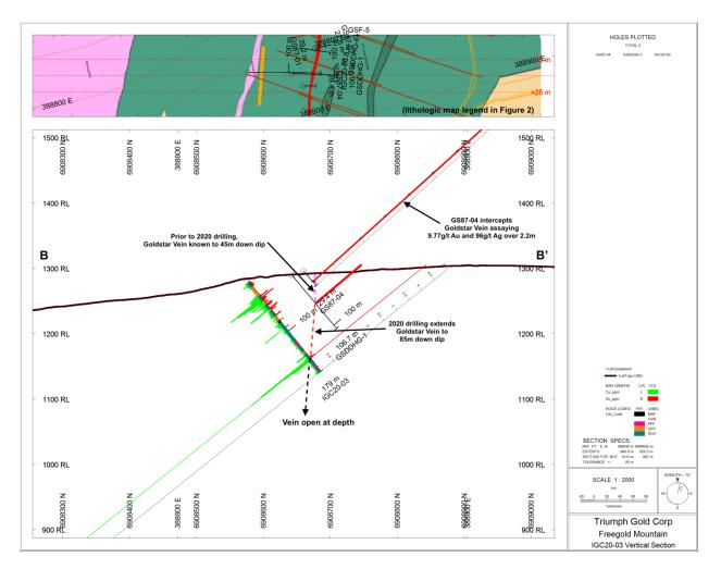
**Figure 4** (Cross-Section B to B' from Figure 2): Cross-section of IGC20-03 with epithermal gold and silver mineralization near surface and intersection of the high-grade Au-Ag-Cu Goldstar Vein, over 85m below its known extent, seen in drill hole GS87-04 at approximately 45 metres depth.
