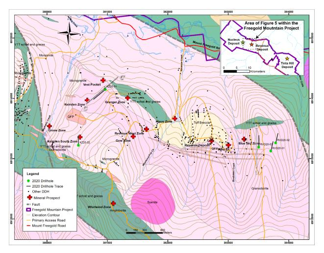
**Figure 5** Plan Map of the Revenue-Nucleus Area. During the 2020 exploration program, two drill holes were completed in the Keirsten area (KZ20-01 and KZ20-02) and three holes were completed in the Revenue East area (RVD20-01, RVD20-02, and RVD20-03).
