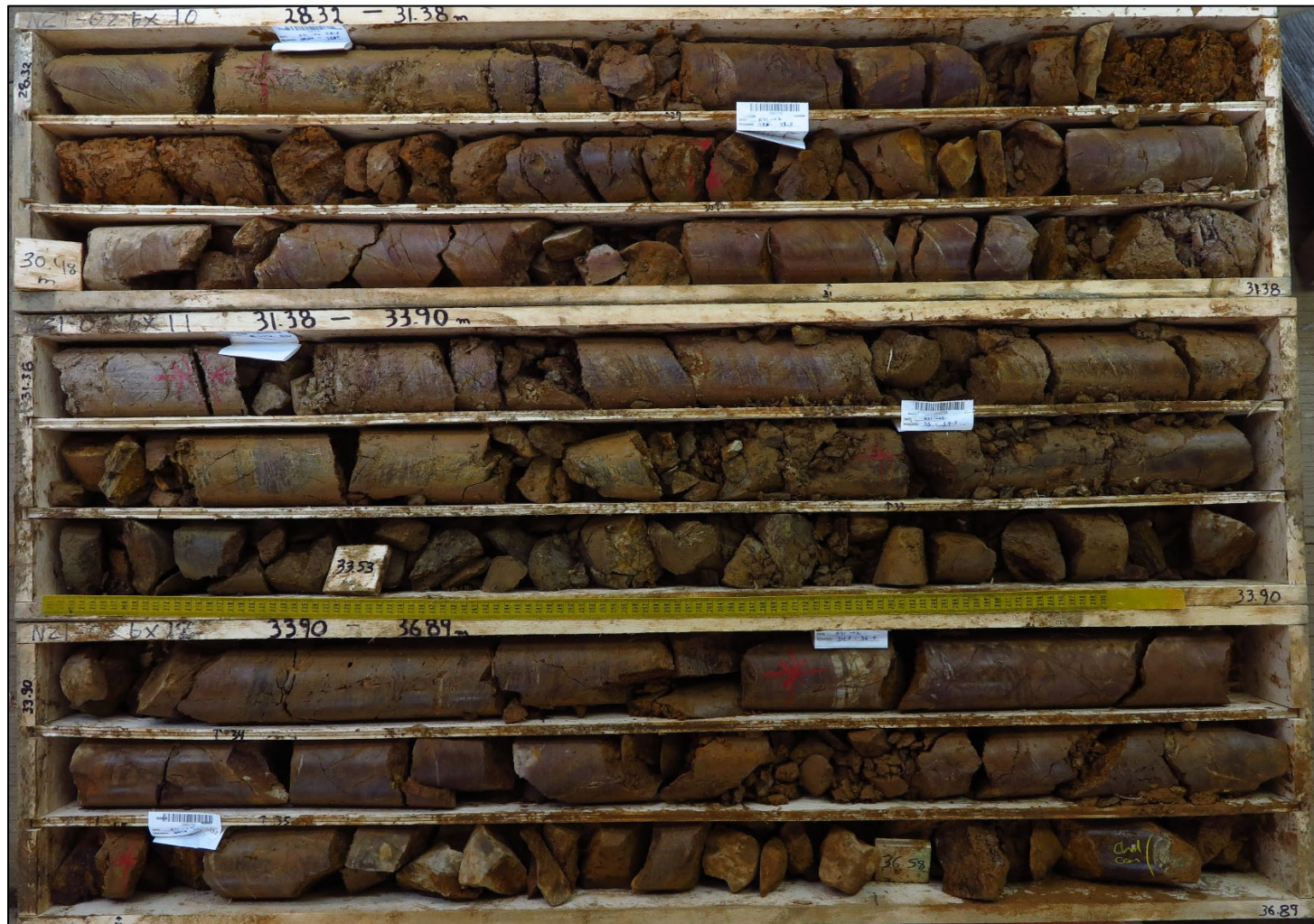
Figure 7. Representative section of core in N21-02 (28.32-36.89m) showing the state of oxidation for the 49.78m oxide gold interval (13.72-63.50m) assaying 0.58 g/t AuEq with an 83% cyanide solubility ratio.
