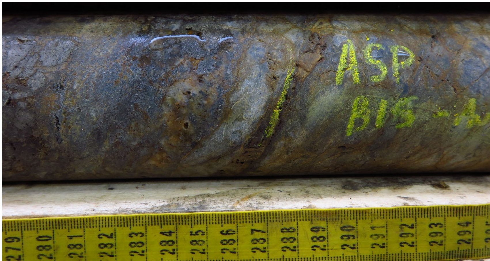
Figure 6. Coarse-grained pyrite-arsenopyrite replacement oriented along the foliation of YTT at 61.50 metres in N21-02 assayed 2.00 g/t Au, 1.2 g/t Ag, and 0.10% Cu (61.50-62.05m).
